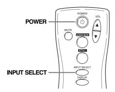
The following is a simple explanation of the procedure for turning the power of the display ON or in STANDBY, and the procedure for selecting the input signal.
